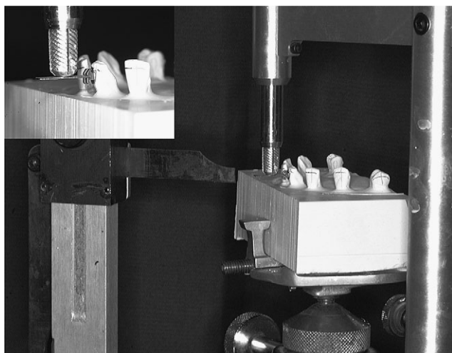
Figure 3 Positioning the bracket using parallelometer.
